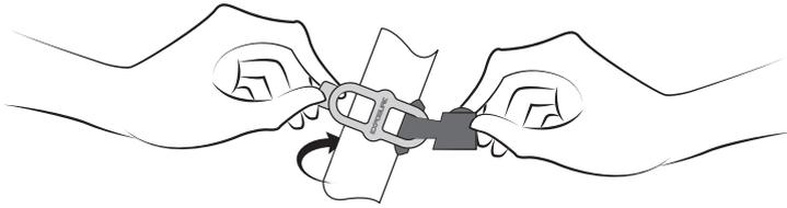
The tab-end fastens onto the lug.
