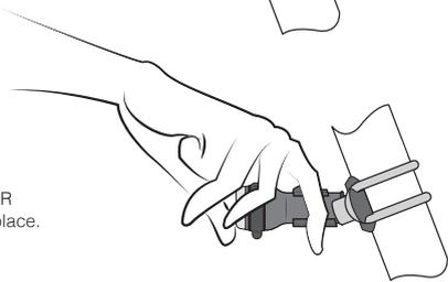
**WARNING:** The TraceR bracket is angled so the light will shine directly back when correctly attached, make sure it is in the correct orientation.
