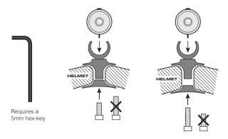
NOTE: The angle of the light can be adjusted by rotating and tilting the ball joint.
