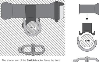
The tab-end of the silicone band fastens on the rear.
