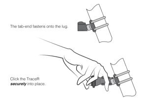
⚠ WARNING: The TraceR bracket is angled so the light will shine directly back when correctly attached, make sure it is in the correct orientation.
