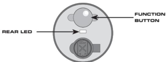
**Bar Lights** – Press and hold the function button until PGM 1 appears on the screen, release. Without delay Press the function button a further 11 times to enter PGM 12, the screen will then show RESET for 1 second.
